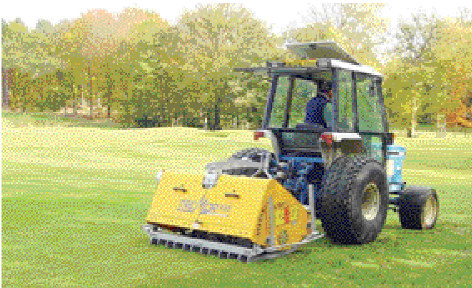
An EarthQuake Model T-155 rotary decompaction unit being used at Duck Hollow Golf Course in Uniontown, Pa.
